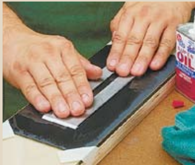
1 Using oil as a lubricant, sand the back of the blade across a piece of silicon-carbide sandpaper.
