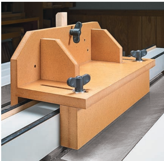
▲ Wide Fence. Slots cut in the horizontal support allow you to adjust the back fence of the jig to fit your rip fence for a smooth sliding fit.
