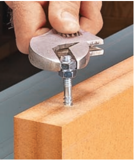
▲ Install Hanger Bolts. Lock two nuts together to make it easy to drive hanger bolts into place.
