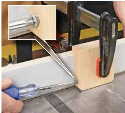
▲ To shorten a board in small increments, use a screwdriver to back out the screw in the stop block a little at a time.
