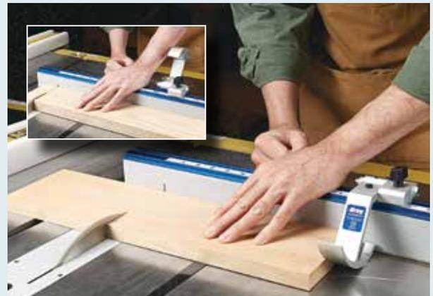
▲ A flip stop allows you to cut other parts to rough length without losing your setting. Just pivot the stop block up and out of the way (inset) to make a cut.
