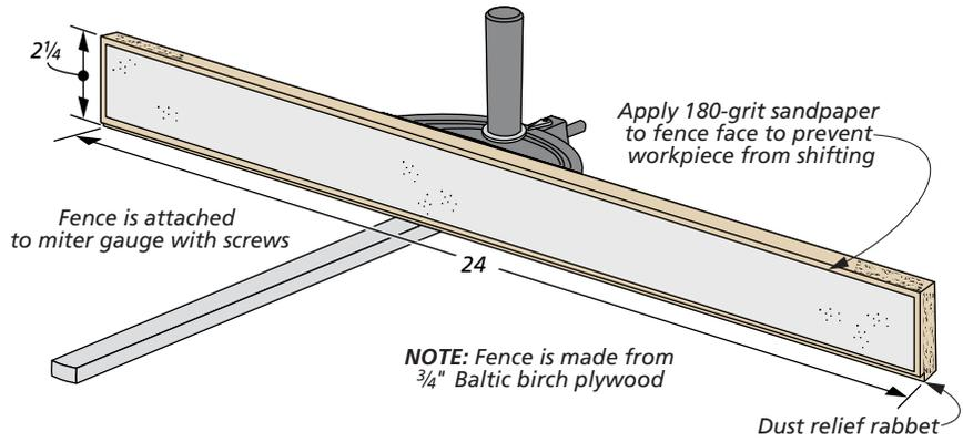
**STOP BLOCK.** Cutting one piece to a given length is relatively easy to accomplish with a miter gauge and a clear layout line. But many projects require cutting several parts to an identical length. Laying out each cut and lining it up
